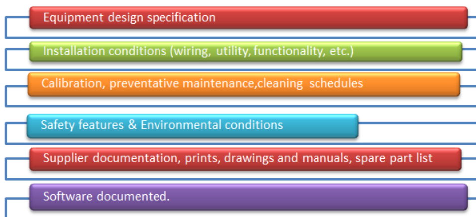
Figure 2: Includes important design specifications for Installation Qualification (IQ) including equipment specifications, installation conditions, calibration, safety features, supplier documentation and software documentation.
