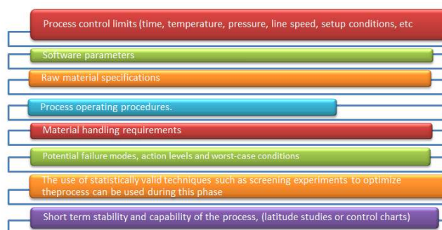
Figure 3: Illustrates the key elements that are considered in the process design phase, namely process control limits, raw material requirements, operating procedures, material handling requirements, failure modes, statistical improvement and process capability analysis.
