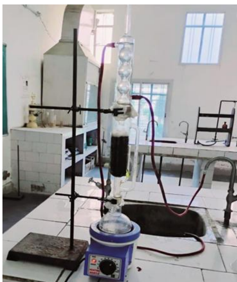
Fig-5: Extraction of Senna occidentalis linn leaf (Soxhlet apparatus)
