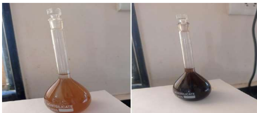
Fig.2 Color Change of Silver Nanoparticle Solution from Light Brown to Dark Brown
