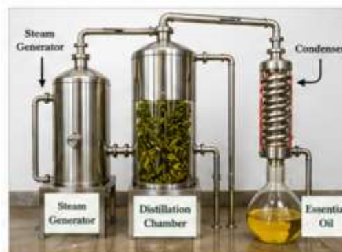
Figure 6. Steam distillation process for extraction of cardamom essential oil.
