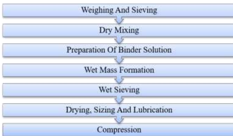
Fig 4. Wet Granulation Method of Tablet Preparation
