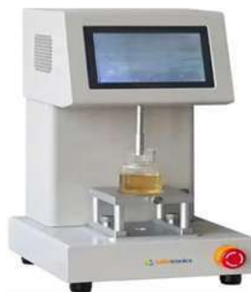
Figure 09: Texture analyzer equipment for quantitative assessment of lip balm hardness and consistency
