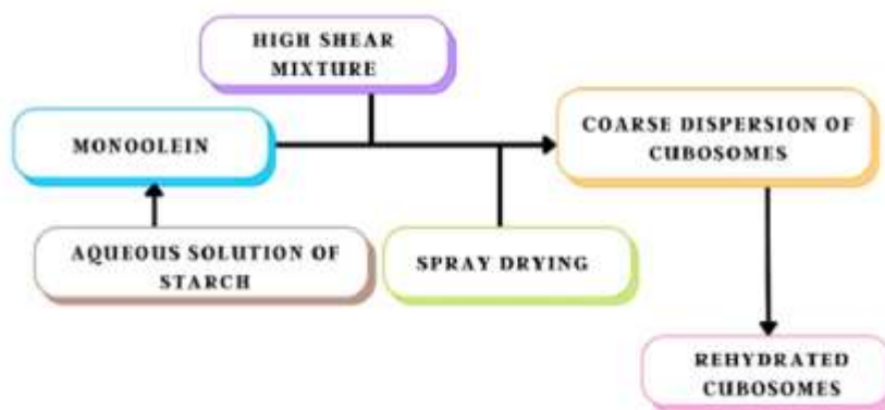
Figure 3: Schematic representation of the preparation of dry powder cubosomes.
