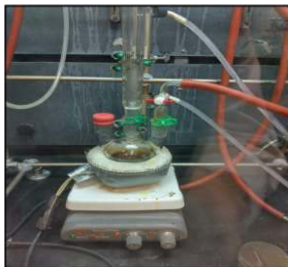
Figure 3: Experimental setup used for the CuAAC synthesis of 4-phenyl-1,2,3-triazole under optimized reaction conditions.
