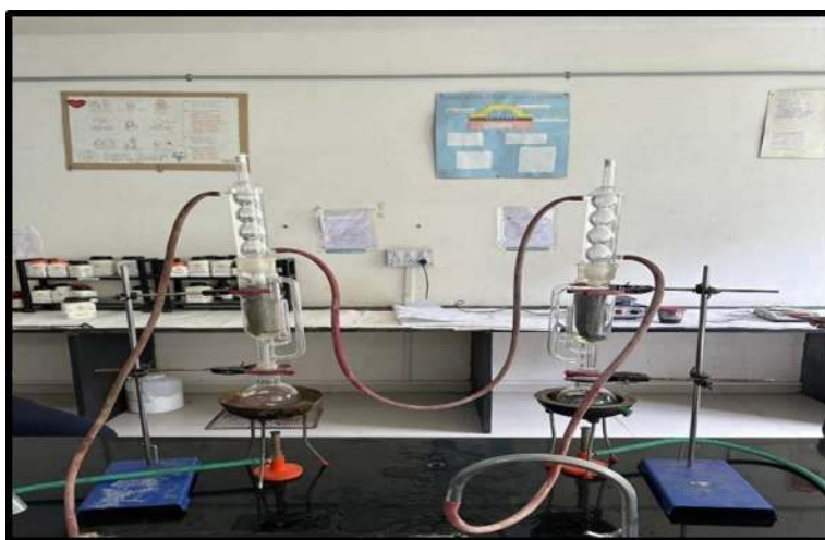
Fig 7.1.2 Extraction of Neem extract
