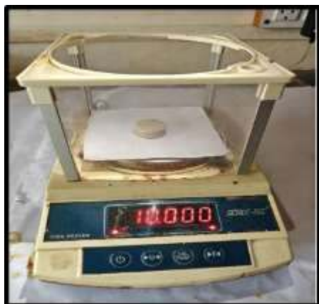
Fig.8.2.1 Weight Variation Test
