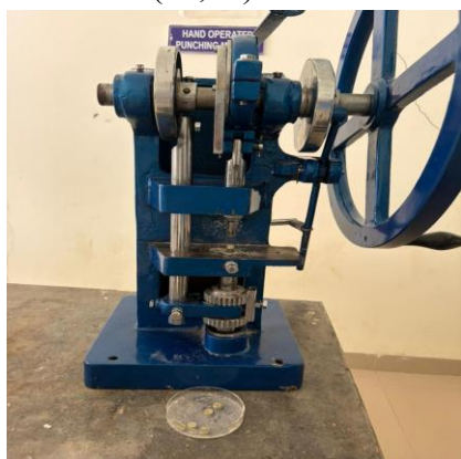
Fig. 7. Single-punch tablet compression machine.
