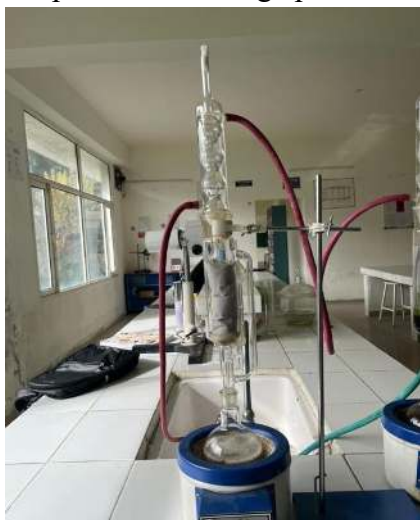
Fig. 2. Hot continuous extraction (Soxhlet) setup.
