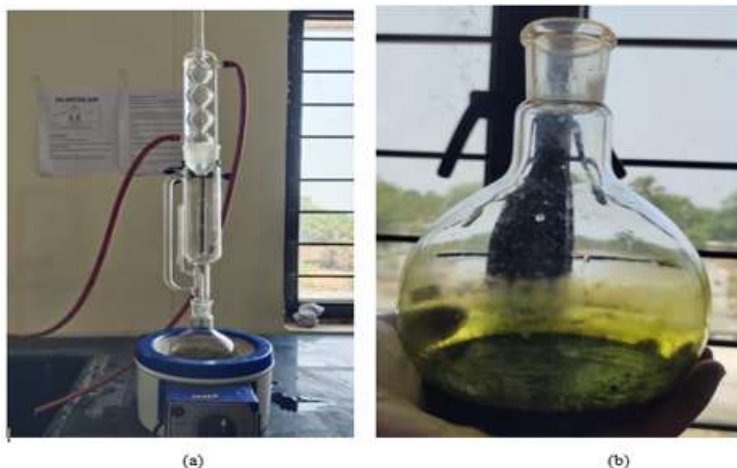
Figure 4: (a) Soxhlet extraction of Murraya koenigii (curry leaves) using ethanol as solvent; (b) Concentrated extract of Murraya koenigii after evaporation showing greenish-black appearance.
