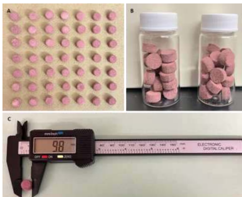
Figure 7 SLS based 3D printed tablets. A) Placebo tablets, B) Tablets in a scintillation vial, and C) Diameter of tablets as measured by vernier calipers.
