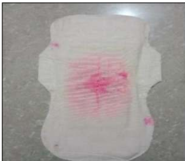
Figure 11: Absorption rate test showing rapid fluid uptake by the developed sanitary napkin.
