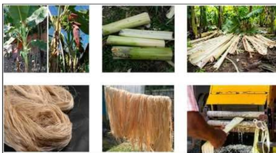
Figure 4: Visual representation of different stages of banana fiber processing, from raw pseudo stem to cleaned, dried, and treated fibers suitable for use as an absorbent material in sanitary napkin formulation.
