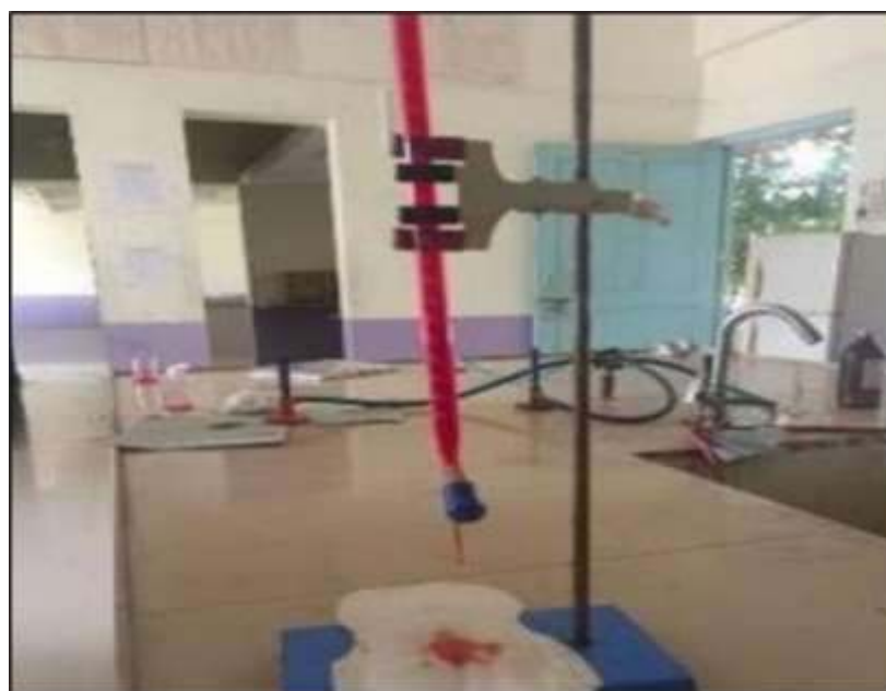
Figure 10: Experimental setup and observation of blood absorption capacity test showing fluid uptake behavior of the developed sanitary napkin.
