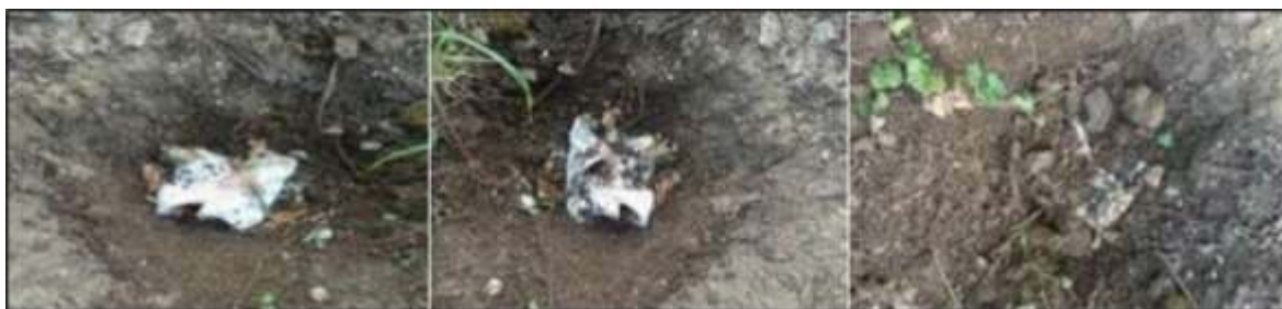
Figure 9: Soil burial degradation study showing progressive breakdown of the developed sanitary napkin over time, confirming its biodegradable nature.
