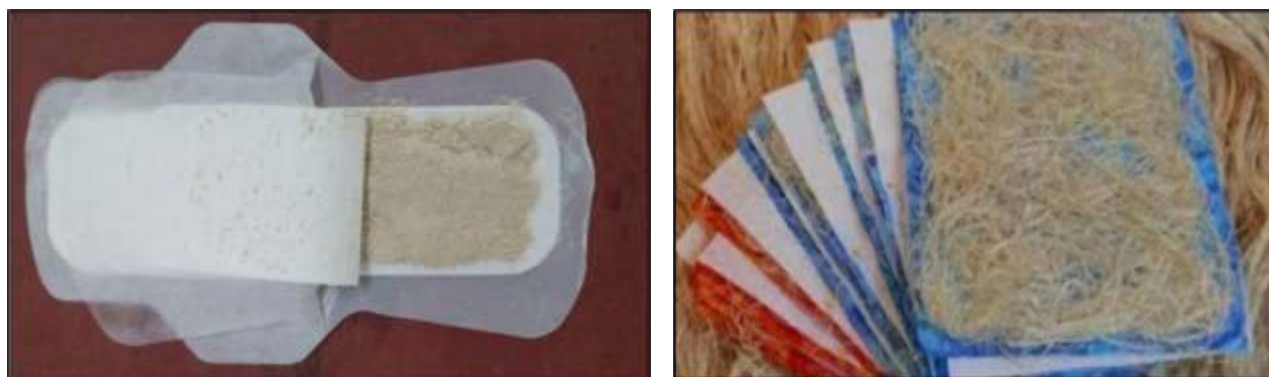
Figure 7: Cross-sectional representation of the developed biodegradable sanitary napkin showing multiple functional layers, including a banana fiber-based absorbent core incorporated with herbal extracts and silver nanoparticles.
