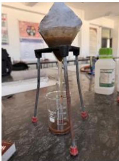
Figure no -02 Extraction setup for Ashwagandha roots Extra
