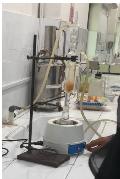
Figure 1: Soxhlet apparatus used during the preparation process.
