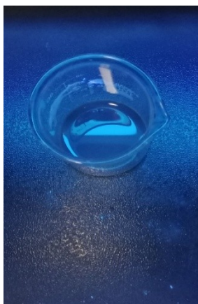
Figure 4b. Fluorescence emission of CDs under UV light at 365 nm (blue emission)
