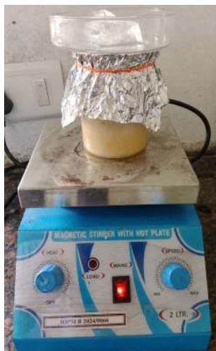
Figure 11. Synthesis setup showing Aegle marmelos seed extract undergoing reflux-assisted heating on a magnetic hot plate stirrer with ice-assisted condensation arrangement.
