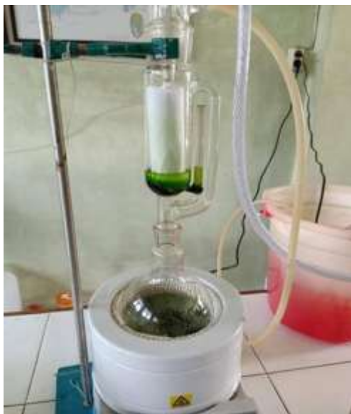
Fig. Soxhlet extraction of Annona squamosa leaf powder
