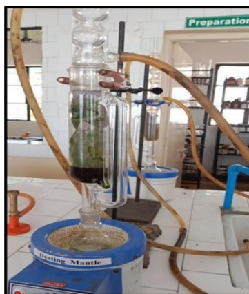
Figure_4 Soxhlet extraction
