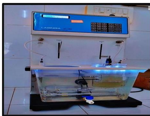
Fig_7 Disintegration Apparatus
