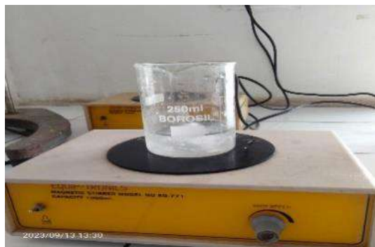
Fig. 4 Gel preparation by using Magnetic stirrer
