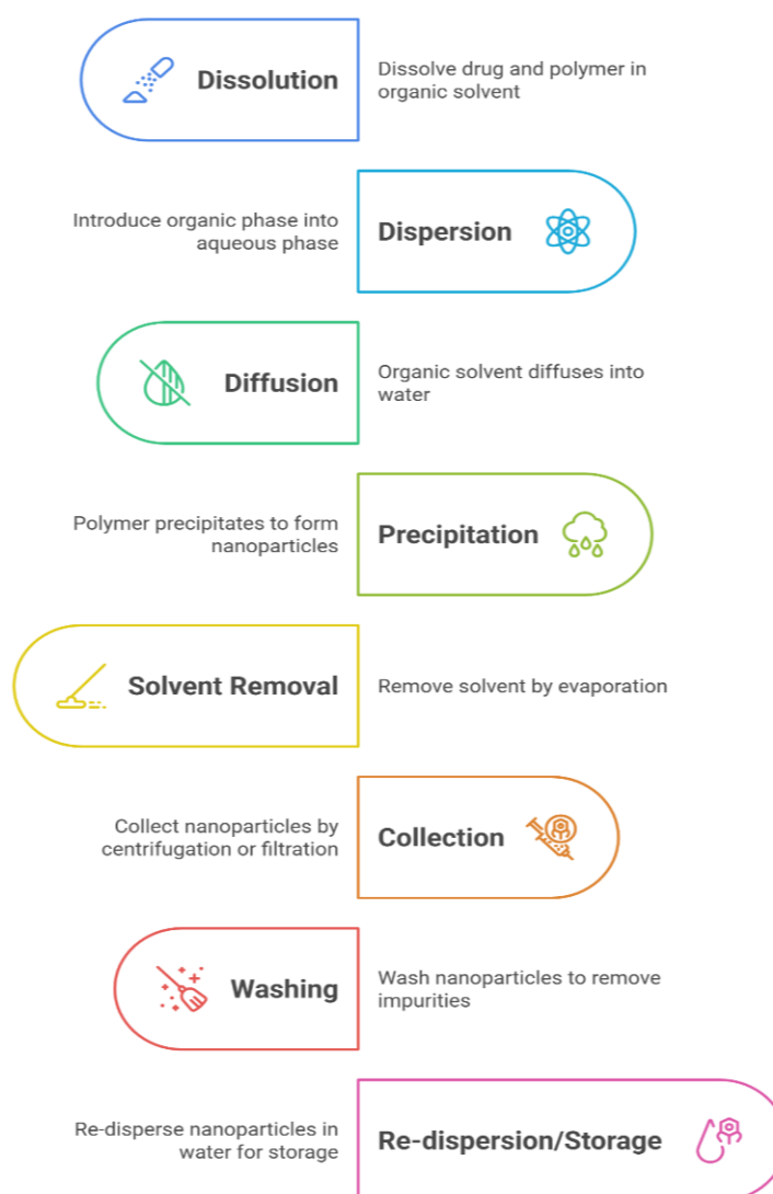
Fig 1.4: - Solvent diffusion method
