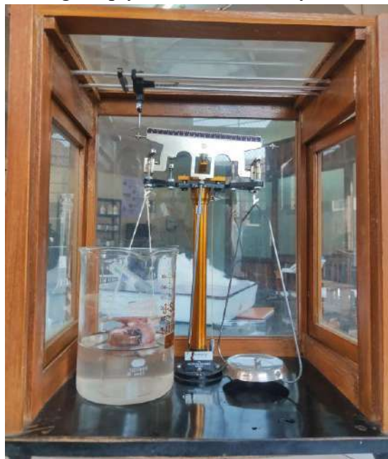
Figure 13. Measurement of bioadhesive strength by physical balance
