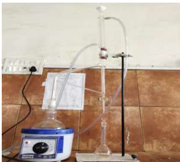
Figure 3.4 Extraction of Oil (Clevenger Apparatus)
