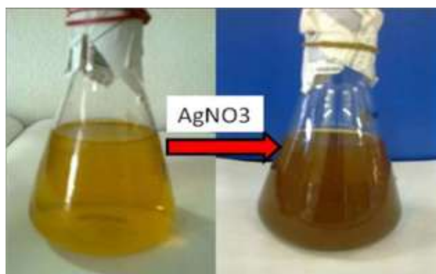
Fig no 02: Colour change of Quercetin before and after addition of AgNO3
