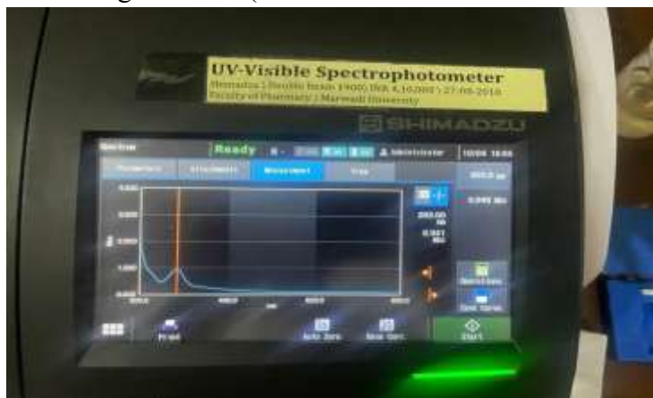
Fig. 2: UV-Visible spectrophotometer (Shimadzu Double Beam 1900) used for the linearity test.
