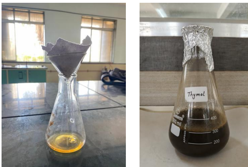
Figure 3. Representative extraction steps: (a) filtration of the distillate; (b) collected thymol (ajwain) oil extract.
