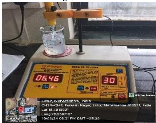
Figure No. 12: photograph showing determination PH of formulation by using Digital PH meter.
