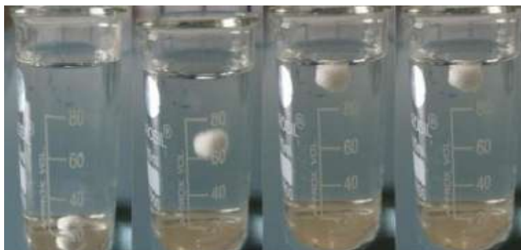
Fig 4: In vitro buoyancy study showing floating behavior of the optimized gastroretentive floating tablet formulation in 0.1 N HCl
