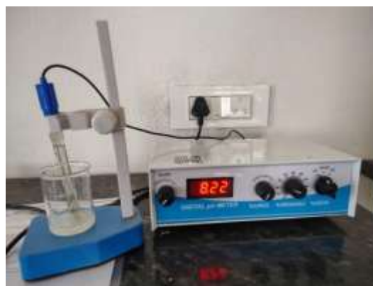
Fig.6:- PH Test Of Soap
