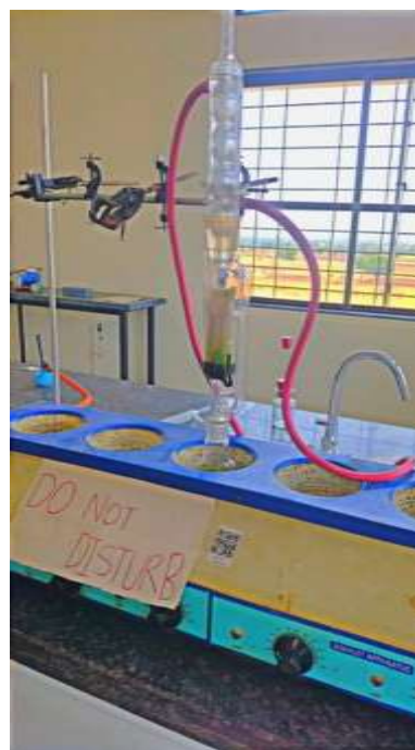
Fig.5 :- Soxhlet Assembly For Extraction
