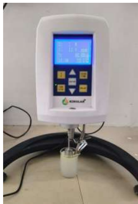
Fig. 4: Determination of viscosity using a Brookfield viscometer
