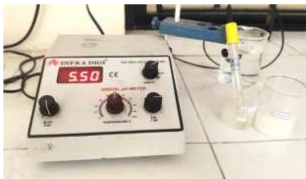
Fig. 5: Determination of pH using a digital pH meter
