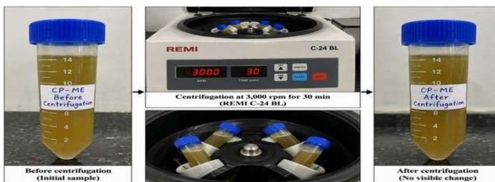
Figure 31: Centrifugation Test of the Prepared Carica papaya Leaf Extract-Loaded Microemulsion.
