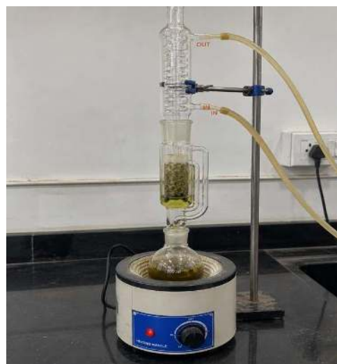
Figure 17: Soxhlet Extraction Apparatus Used for Carica papaya Leaf Extraction.
