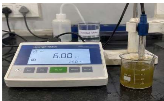
Figure 26: Measurement of the Initial pH of the Prepared Carica papaya Leaf Extract-Loaded Microemulsion.
