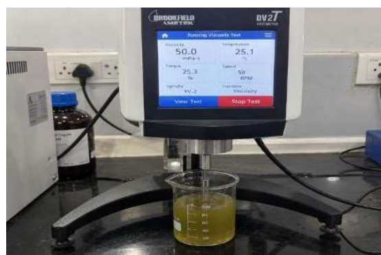
Figure 27: Viscosity Measurement of the Prepared Carica papaya Leaf Extract-Loaded Microemulsion Using a Brookfield DV2T Rotational Viscometer.
