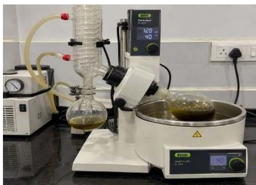
Figure 19: Concentration of Carica papaya Leaf Extract Using a Rotary Evaporator.
