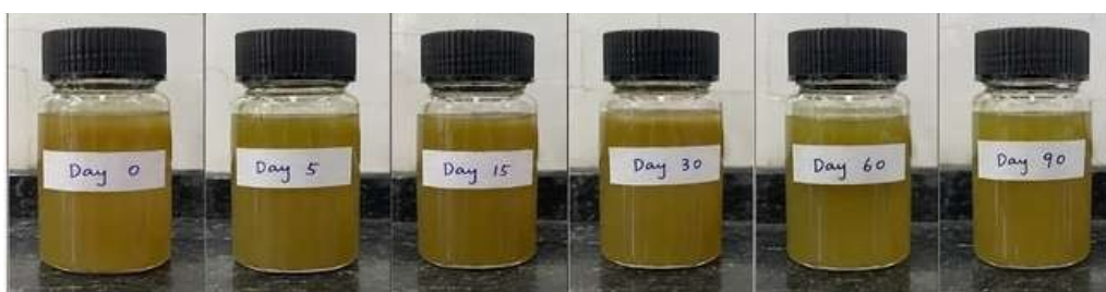
Figure 30: Physical Appearance and Stability Assessment of the Prepared Carica papaya Leaf Extract-Loaded Microemulsion During 90-Day Room-Temperature Storage.
