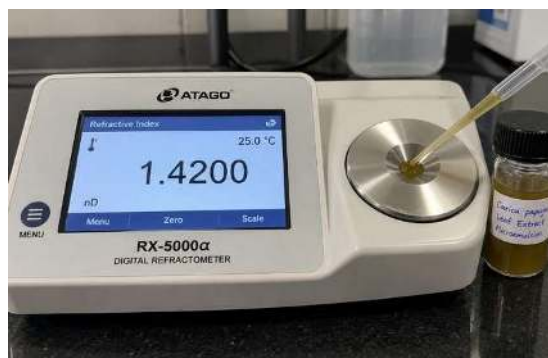
Figure 29: Refractive Index Measurement of the Prepared Carica papaya Leaf Extract-Loaded Microemulsion.
