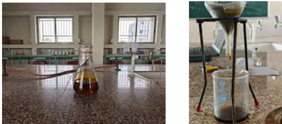
Figure 5: Extraction procedure showing maceration flask with hydroalcoholic extract (top) and filtration through muslin cloth (bottom).
