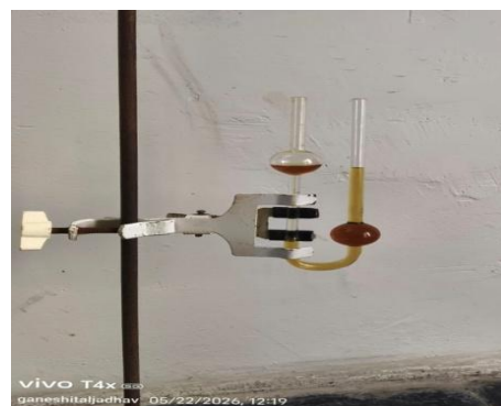
Fig.8.ostwald viscometer (viscosity determination)
