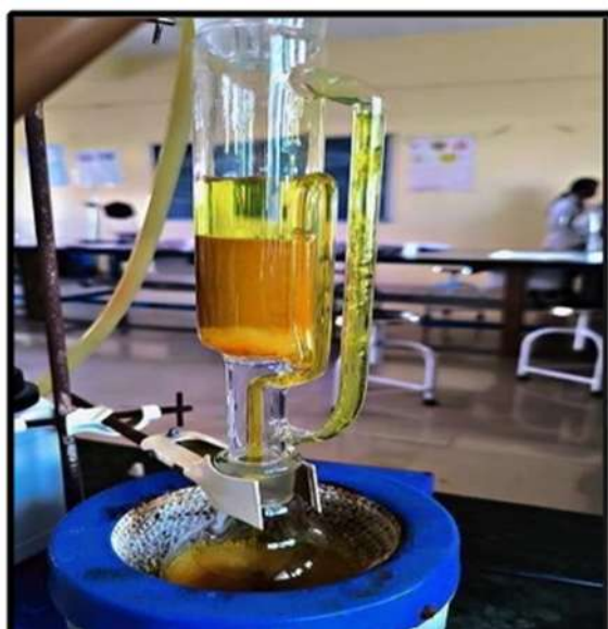
Soxhlet Extraction of Curcumin
