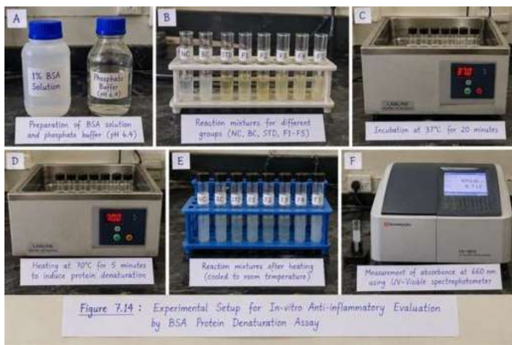
Figure 6. Experimental Workflow for In-vitro Anti-inflammatory Evaluation by the BSA Protein Denaturation Assay
