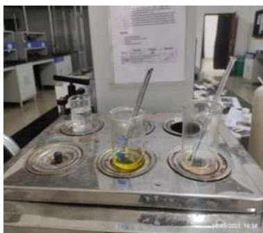
Figure 40: heating on waterbath
