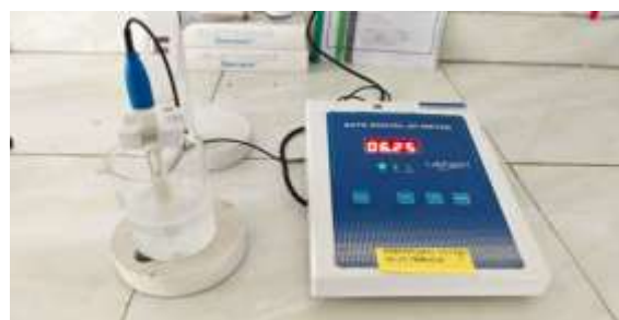
Fig no.10: - pH testing of Hydrogel using pH meter
