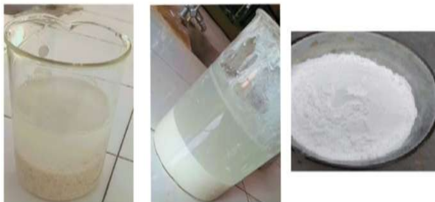
Fig.5:- Rice soak in water. Fig.6:- Separation of Rice starch from water. Fig.7:- Starch
