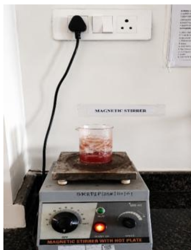
Fig. 5: Preparation Of Extract Stock Solution For Phytochemical Test On Magnetic Stirrer
