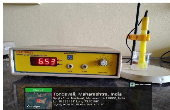
Figure 9. pH measurement of the lip balm dispersion using a digital pH meter.
