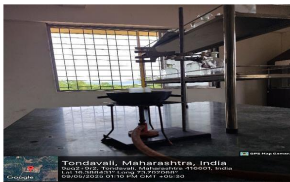
Figure 11. Melting-point determination of the lip balm.
