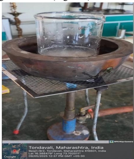
Figure 5. Deproteinisation of the demineralised shell residue in dilute sodium hydroxide under gentle heat.
