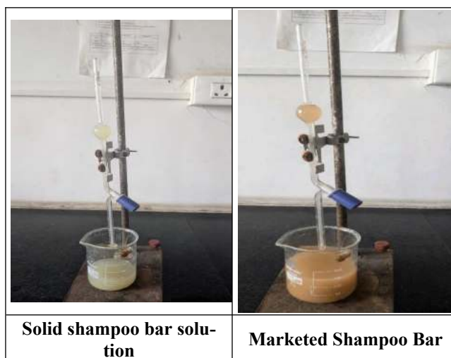
Figure 39: Drop count test for water and solid shampoo bar
