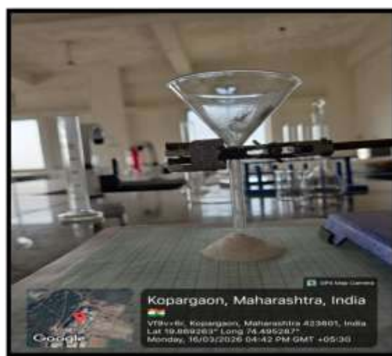
Fig. No. 08 Angle of Repose
