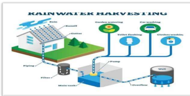
Figure12: Rain water harvesting system
