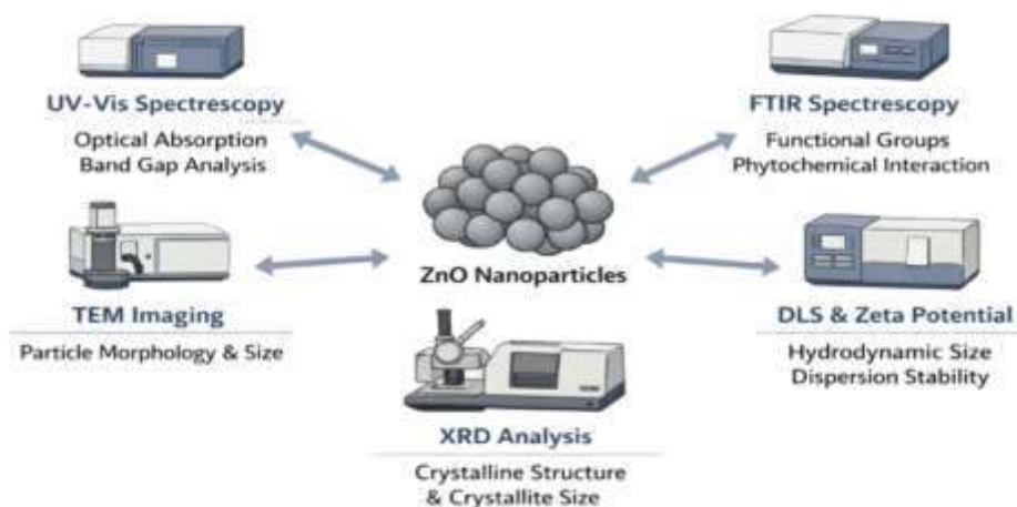
Figure No.2: Analytical tools employed for physicochemical evaluation of biosynthesized ZnO nanostructures.
