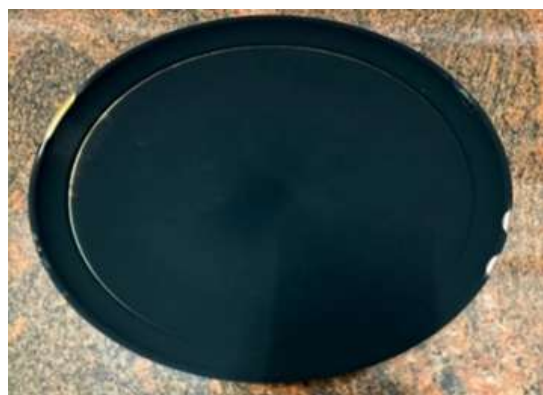
Fig.no: 11 Black soot is obtained on copper
