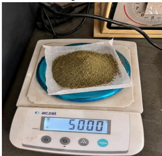
Figure 4. Weighing of powdered plant material prior to Soxhlet extraction (50.00 g).
