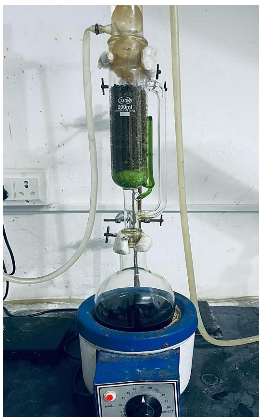
Figure 5. Soxhlet extraction apparatus used for solvent extraction of leaves and stem.
