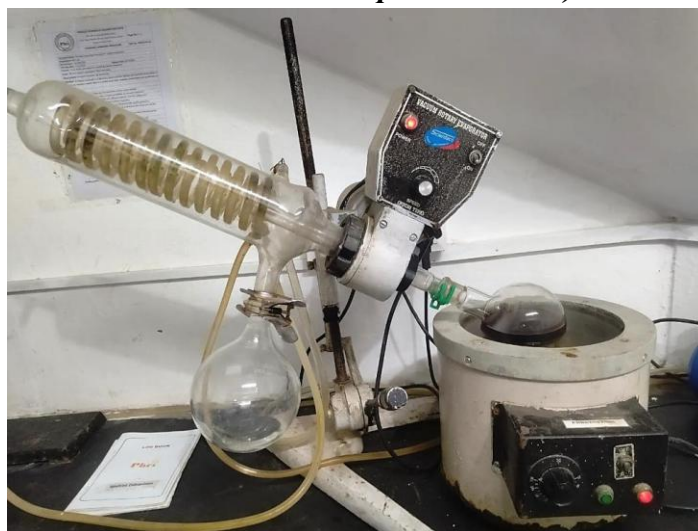
Figure 6. Rotary vacuum evaporator (Rotavap) used to concentrate the crude extracts.
