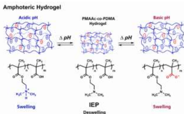
Figure 7: pH-Responsive Swelling and Deswelling Behaviour of Amphoteric Hydrogels Under Different pH Conditions
