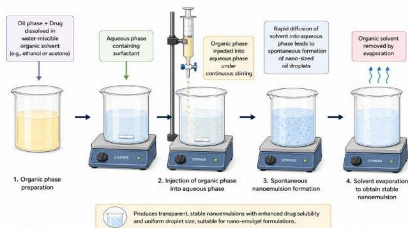
Figure 9. Solvent displacement (spontaneous emulsification) method: injecting a drug-loaded organic phase into an aqueous surfactant phase drives spontaneous nanodroplet formation as the solvent diffuses out and evaporates.
