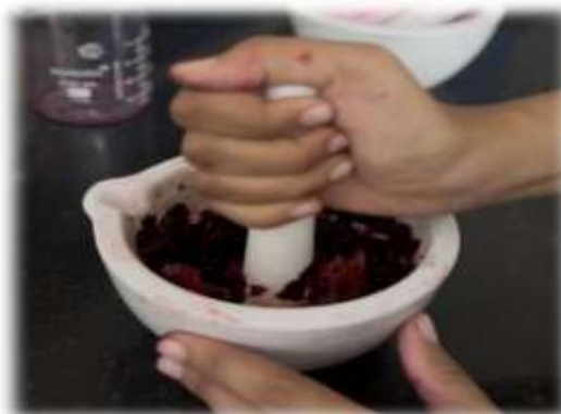
Figure 1: Beetroot grinding for pigment extraction
