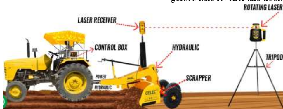
Fig. 2. How a laser land leveller works
