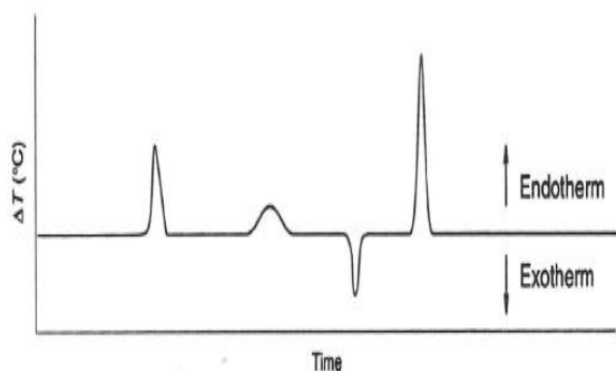
A hypothetical DSC thermogram showing the changes that might occur upon heating a sample.
